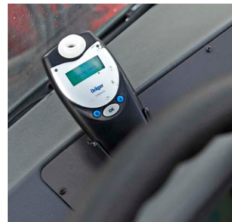
To increase workplace safety the machine can be fitted with alcohol interlock.
