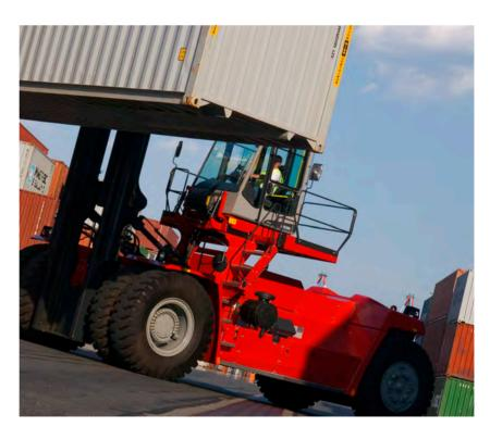
Designed to have great horsepower to weight ratio the Kalmar DCF generates higher capacities with very stable axle loadings.
