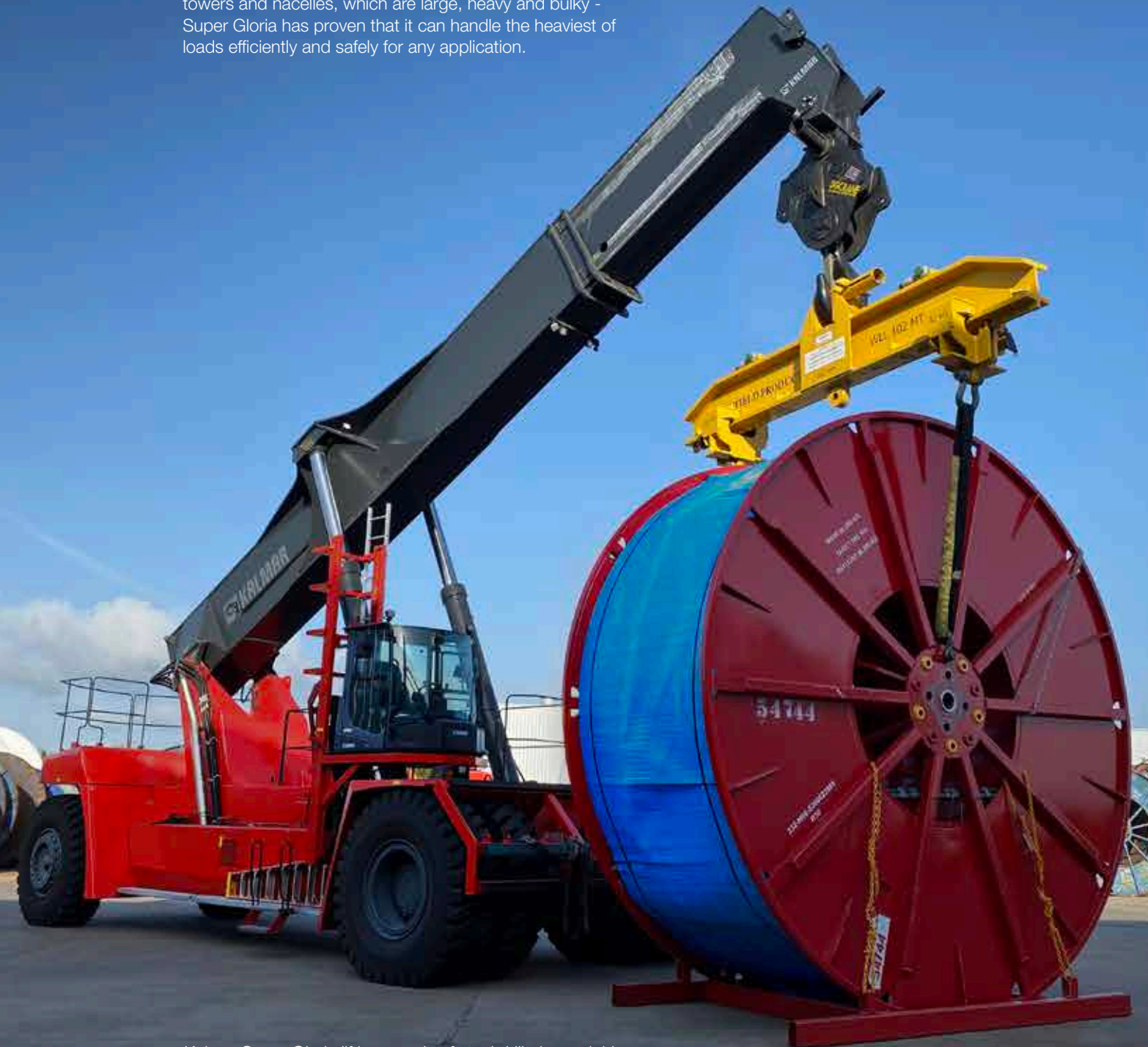
Kalmar Super Gloria lifting spools of steel drill pipe weighing over 165,000 lbs for an oil company in Houston.
