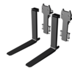
Quick change system with separate carriers for each fork
